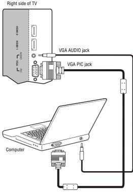
3 Connect an audio cable to the VGA AUDIO jack on the right side of your TV, then connect the other end of the cable to the AUDIO OUT jack on the computer.
